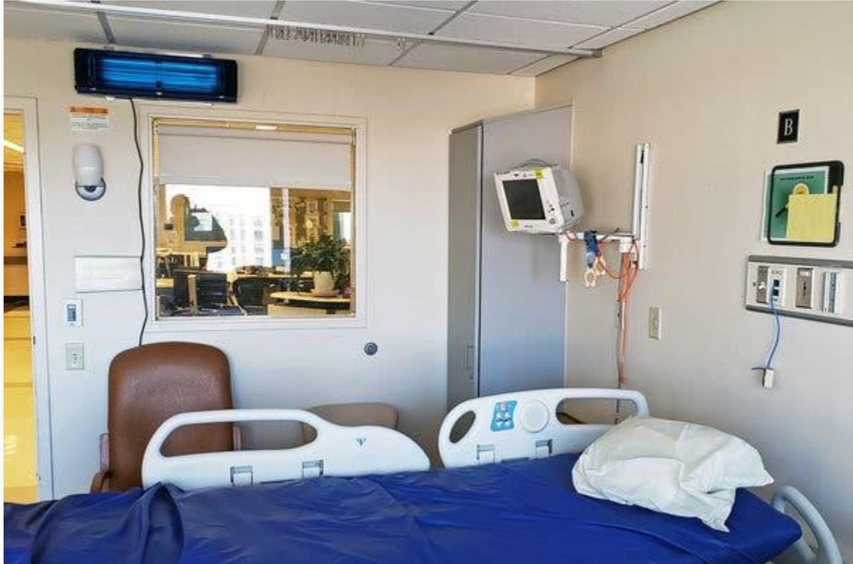
A patient room with an ultraviolet light, upper left, installed to zap pathogens. The practice, called upper-room ultraviolet germicidal irradiation, was first tested in the earlier half of the 20th century.
